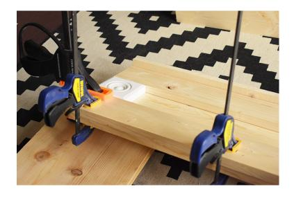
5. Glue a 1" x 4" x 4' board to the 1 x 12, butted up against the wood rosette. Clamp together until the glue is dry.
