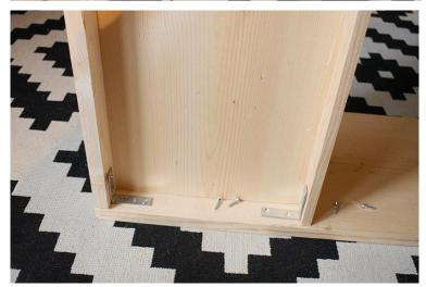
9. Stand your fireplace up on top of your last 1 x 12 board. Align the edge of the fireplace leg to the back of the 1 x 12 board. Use L-brackets and the screws they came with to attach the fireplace to the floor board. Use two L-brackets on each leg.
