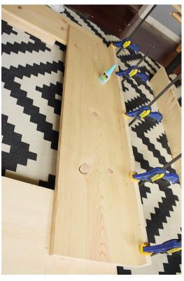
2. Glue a 1"  $\times$  2"  $\times$  4' board to the last 1  $\times$  12 board, as shown. This board will be the front piece that sits on top of your legs. Clamp together until dry.
